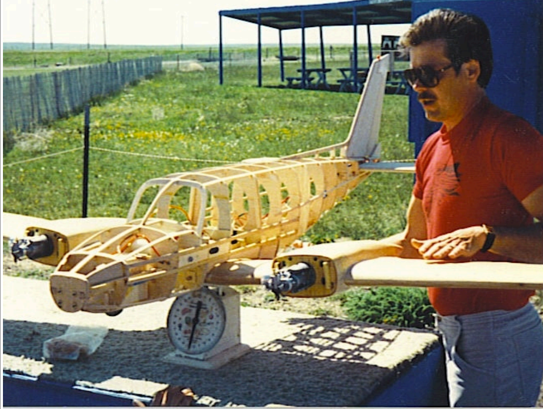
Mark Burr's First RC Airplane Build - He scratch built this Cessna 340
